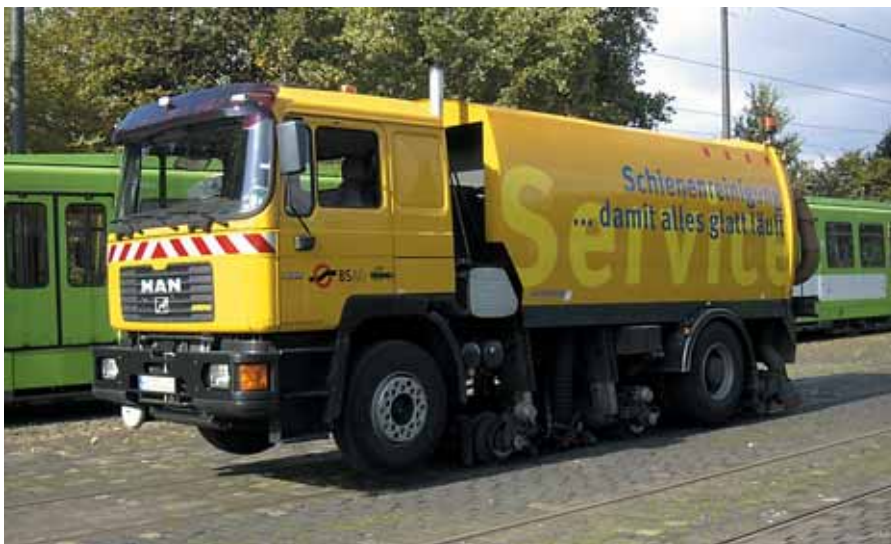
Practically all Tramlub lubricants can also be applied with special "Hi-Rail" service vehicles.
